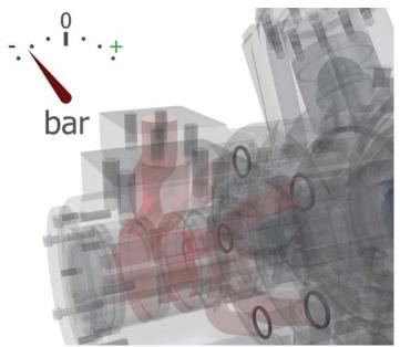
Cavitation can occur due to many different factors. Although it is not possible to make the HMB motor resistant to cavitation, certain features can be added to improve the motor's resistance to short periods of lost port pressure.
